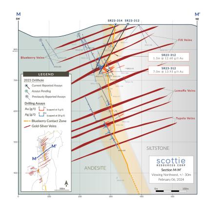
Figure 2: Cross-section highlighting the recent intercept in SR23-312 and 314 relative to previously release intercepts of the vein structures.
