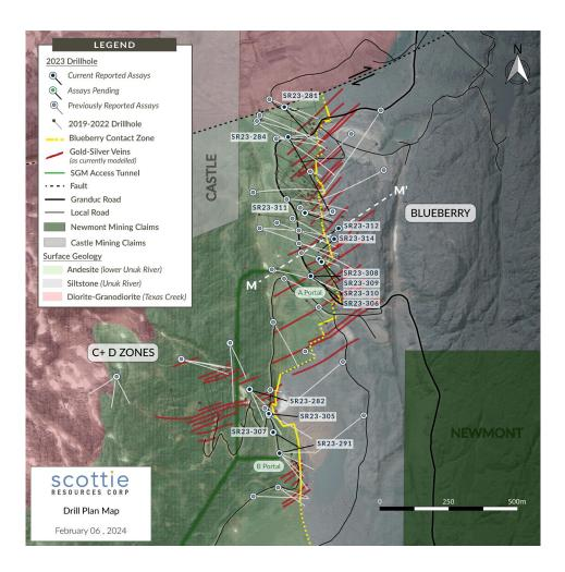
**Figure 1:** Overview plan view map of the Blueberry Contact Zone, illustrating the locations of the reported drill results, cross-section (Figure 2), and the distribution of the modelled sulphide-rich cross-structures.
