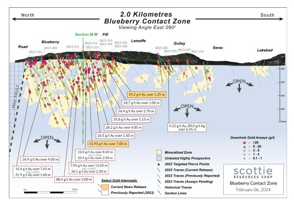
**Figure 3:** Segmented vertical long section of the Blueberry Contact Zone illustrating the distribution and status of drilled targets from the 2023 season and the reported results thus far, relative to intercepts from previous drilling campaigns.
