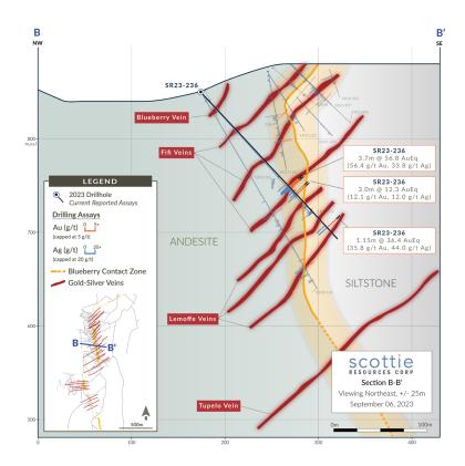
**Figure 4:** Cross-section displaying vein and contact style intercepts highlighted by the recent intercept in SR23-236 located in the main portion of the Blueberry Contact Zone.
