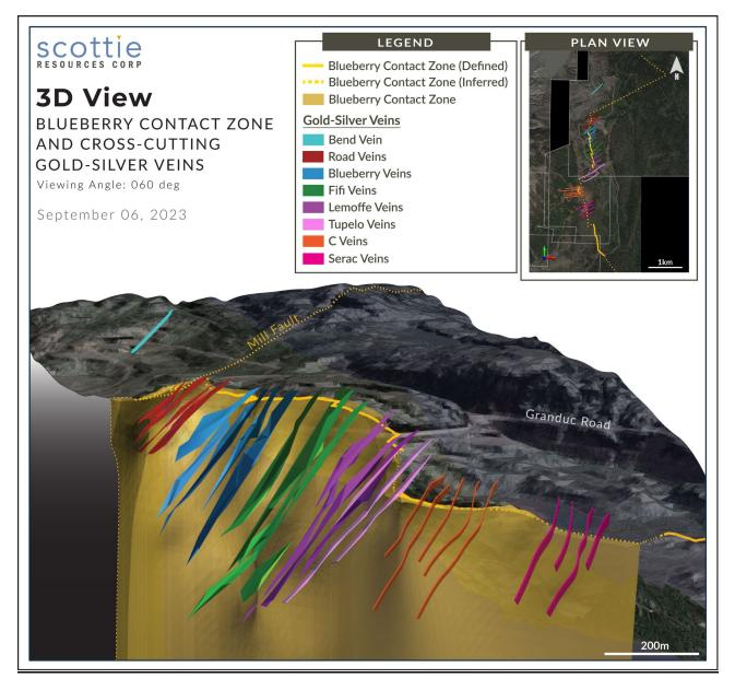
**Figure 1:** Conceptual model for the interaction between SW-trending sulphide-rich cross-structures and the vertical N-S oriented lithological contact that defines the Blueberry Contact Zone.
