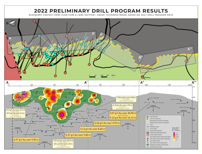
**Figure 1:** Segmented vertical long section of the Blueberry Contact Zone and plan view illustrating the distribution of the sections. Highlighting the distribution and status of drilled targets from the 2022 season and the reported results thus far, grade contour model was created from pre-2022 drilling of the structure.
