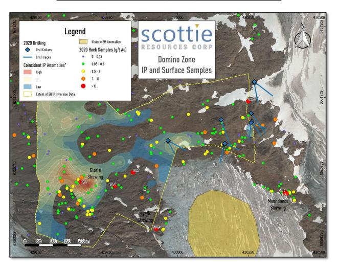
**Figure 1:** Plan view map of the Domino Zone illustrating the locations of the 18 holes drilled during the 2020 field season, and distribution of grab samples. \*IP anomaly layer is a composite heat map comprised of corresponding conductivity highs and resistivity lows derived from a 2D inversion of IP data at a 50 m depth.
